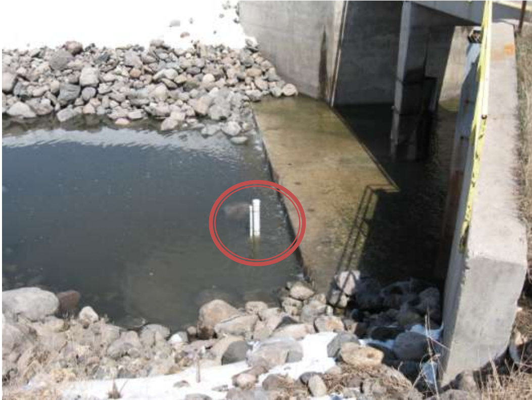
A2 Eureka Manta Multi-parameter sonde and HOBO Water Level Logger pipes.
